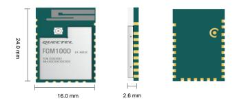
FCM100D is a cutting-edge MCU Wi-Fi and Bluetooth module launched by Quectel. It boasts a high-performance processor with a frequency of up to 120 MHz and supports IEEE 802.11b/g/n protocol and Bluetooth 5.2. The module features built-in 256 KB RAM and 2/4 MB flash, ensuring efficient performance. In addition, it complies with WPA-PSK, WPA2-PSK and WPA3-PSK security standards.
